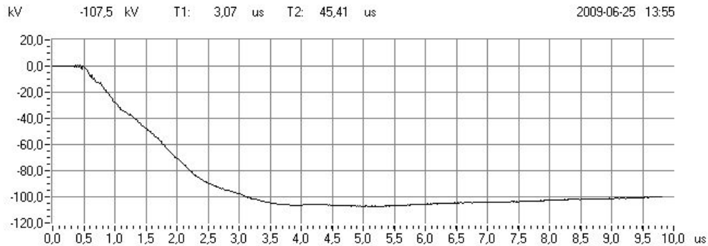
Fig. 5: Waveshape 70870224 Elsewedy -55% of test voltage
